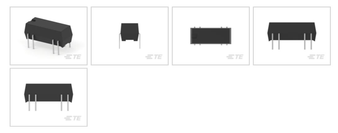
Contact Voltage Rating: 24 VDC Signal Relay Coil Power Rating (DC): 50 mW Signal Relay Mounting Type: Printed Circuit Board Signal Relay Terminal Type: PCB-THT Signal Relay Coil Voltage Rating: 15 VDC
